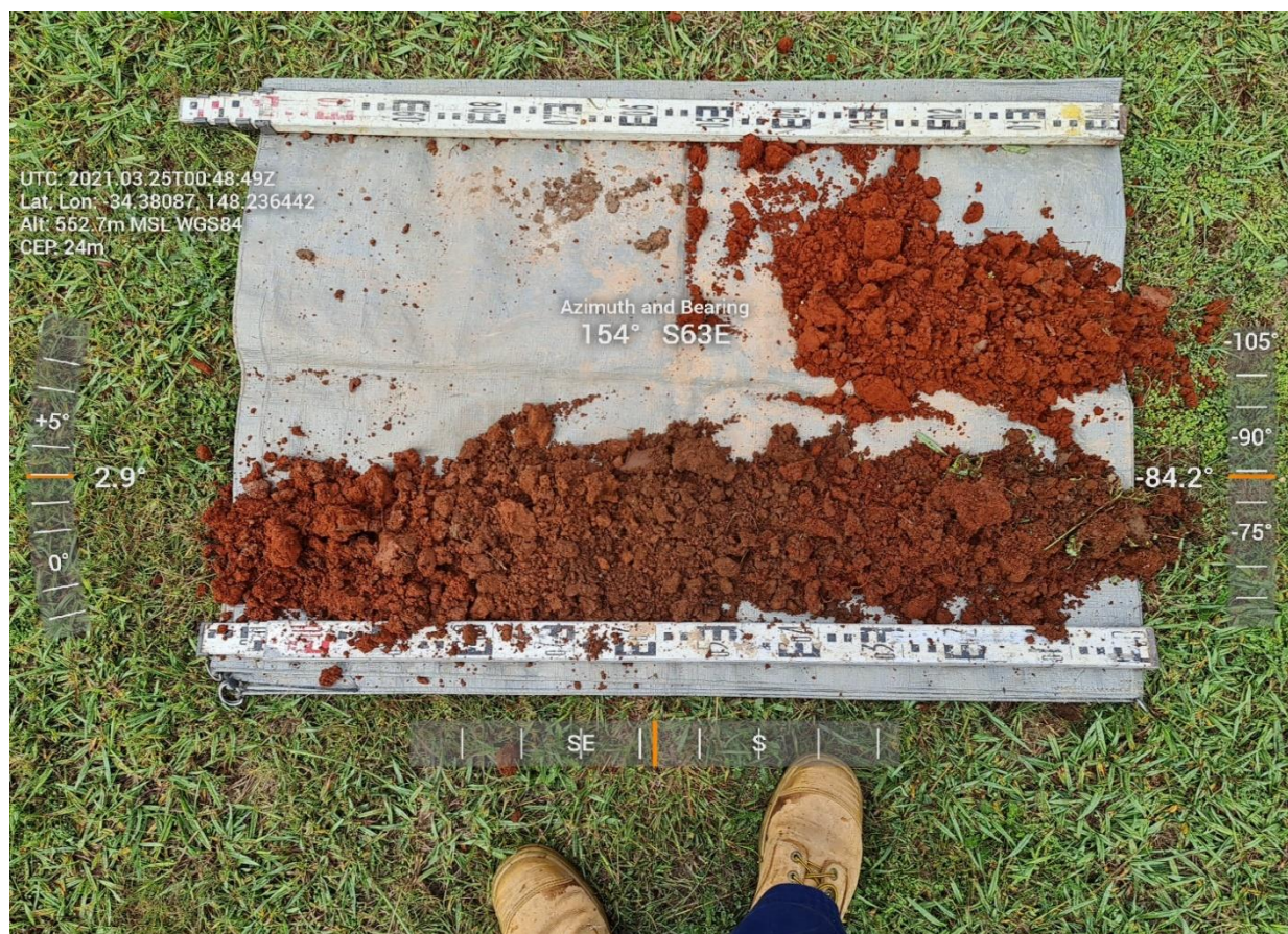
Figure 9: Soil profile – effluent dispersal area
